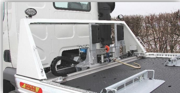
DEPLACEMENT LATERAL PAR VERIN MOVING LATERALLY BY HYDRAULIC CYLINDER
