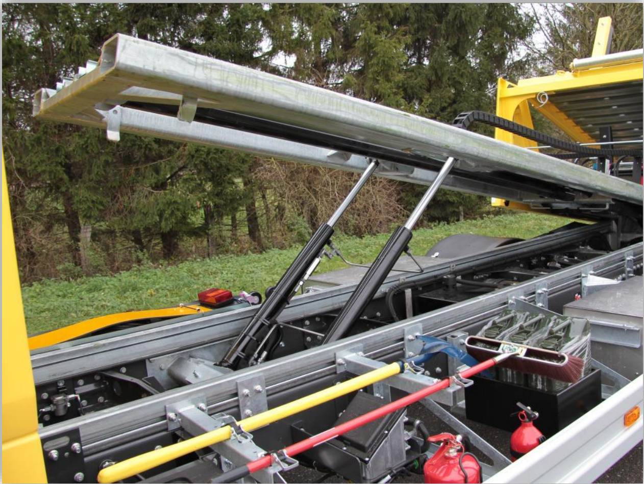
FAUX CHASSIS ET BASCULEUR GALVANISES / HELPERFRAME AND TILTING FRAME FULLY GALVANIZED
