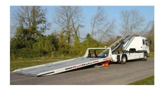
**2008** saw the launch of a new range of sliding trays. The result is a range of standardised sub-assemblies that are easy to fit to all types of chassis. The wiring harness has a directed connector system that immediately identifies any faults, leaving scope for additional options not provided for at the time of construction.
